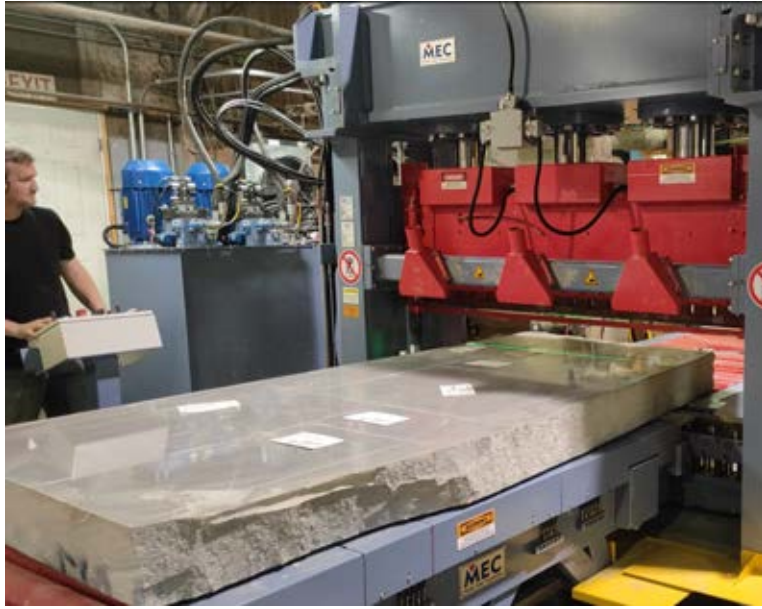
Tesmo H-frame Split-Face splitter for wide full slabs.
